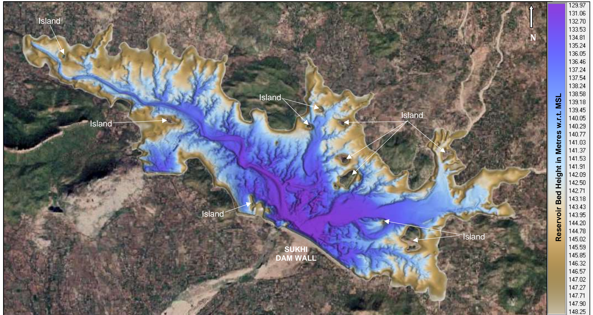
Figure 5.1: Image showing gridded SBES Bathymetry and topography data (superimposed with satellite imagery) of reservoir bed heights in metres from lowest bed level to FRL
